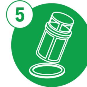
Remove build-up of food debris from the filters at regular intervals
