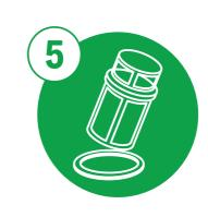
Remove build-up of food debris from the filters at regular intervals
