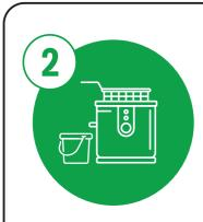
Allow the fryer to cool down and drain into a suitable empty container
